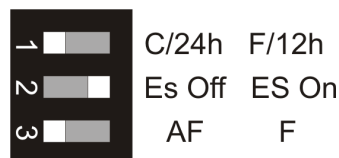
TH115-AF Thermostat DIP Switches
